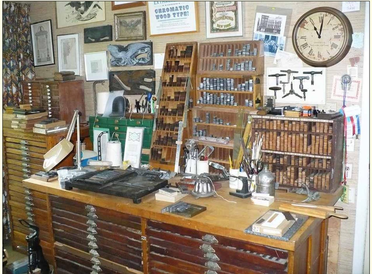
The workbench where type is set and forms made up. Type cases below. At the left, framed above the bench, are a leaf printed by Caxton (*Canterbury Tales*) and a snippet of Gutenberg (*the Catholicon*.)
