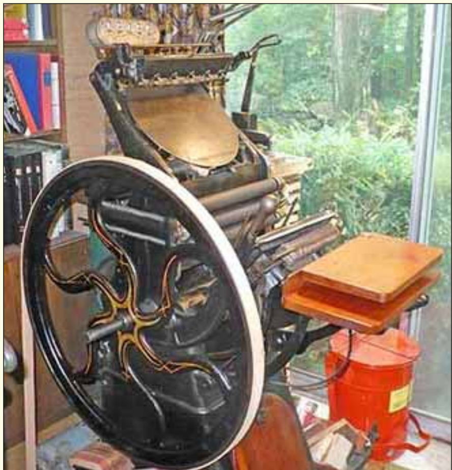
The work horse of the Saxe print shop, the Pearl press, complete with counter, fountain, safety curtain and brake.
