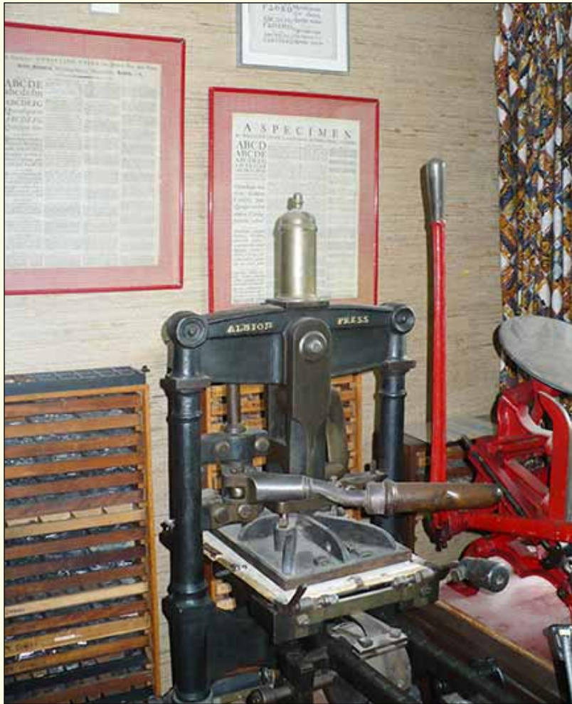
Another corner of the shop, showing quarter cases of spacing, the Albion and Pilot presses. Framed above are broadside type specimens by Joseph Fry (1785) and William Caslon (1734.)
