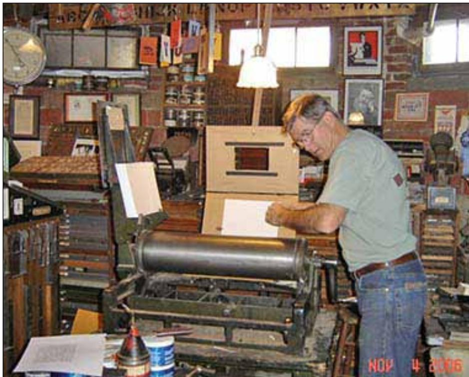
Rick von Holdt and his POCO proof press. The blanket and packing have been removed from the cylinder in this photograph because Rick was using a tympan and frisket setup that was built for him by Neil Giroux. This is very much like printing on a handpress, but using a cylinder to create the impression.
