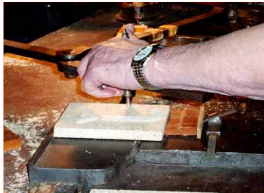
Left, a punch press used to stamp designs into blocks for boders. Above, a pattern is being traced while cutting a letter on the pantograph.
