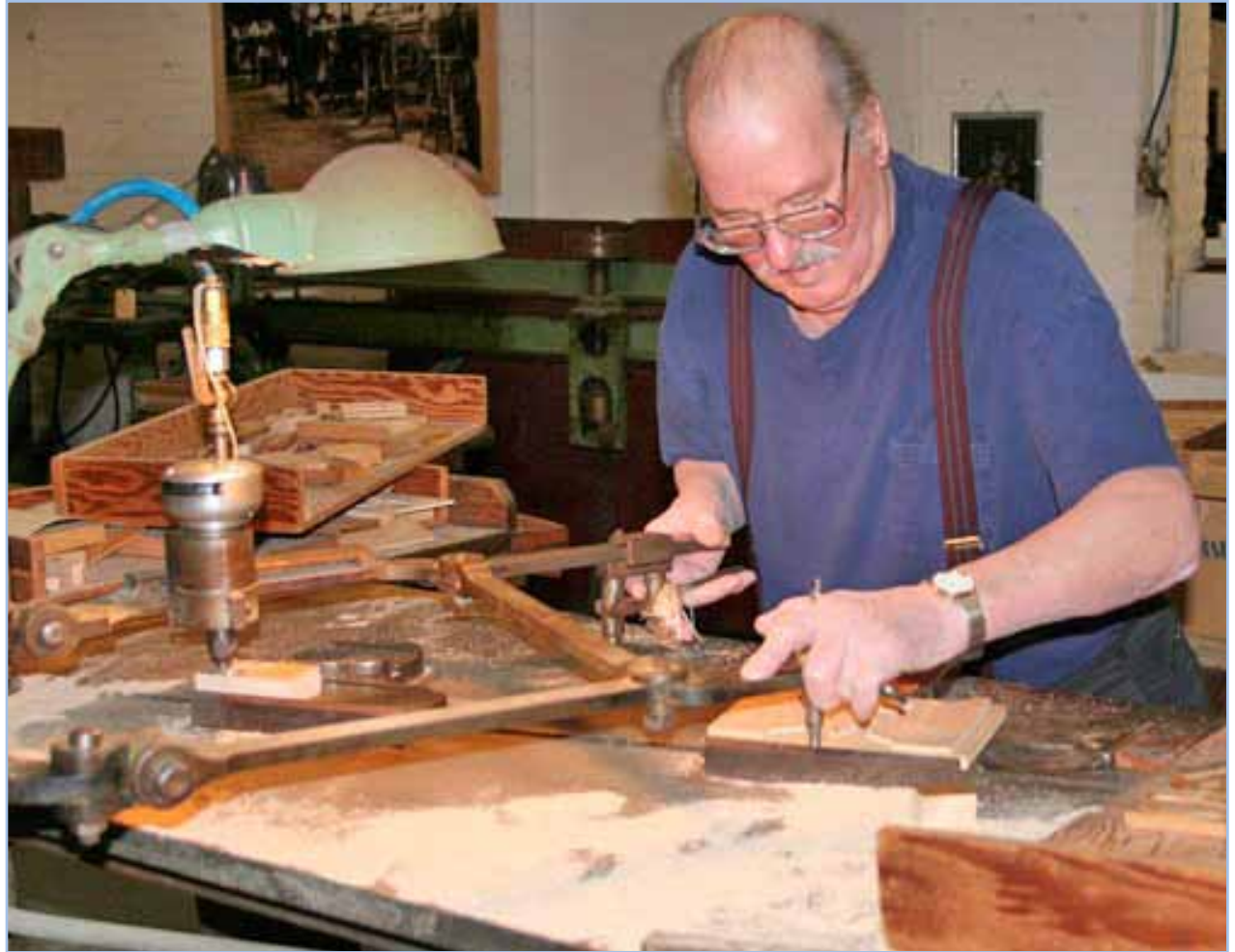
Norb Brylski demonstrates the pantograph, a device that cut wood type from plywood patterns.
