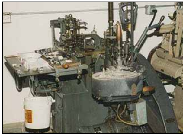
This is an English Monotype Display Caster, popularly known as an "Orphan Annie."
