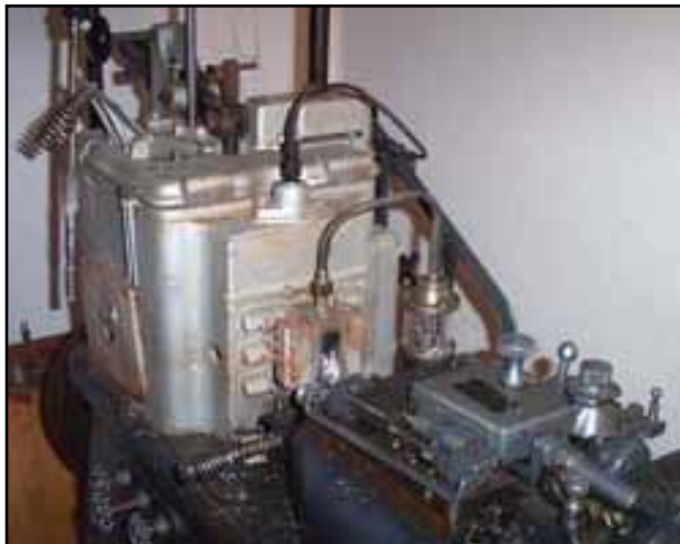
An Elrod stripcaster—my first hot metal machine.
